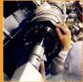
Positioning of FE300 on top of see through glass of vacuum chamber
